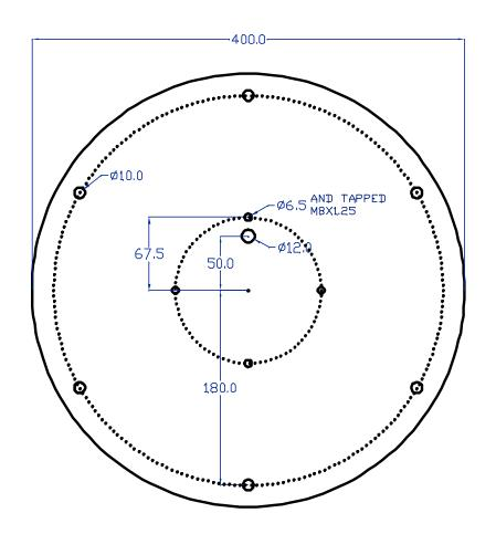
All dimensions in mm Material: 5/16" mild steel plate
